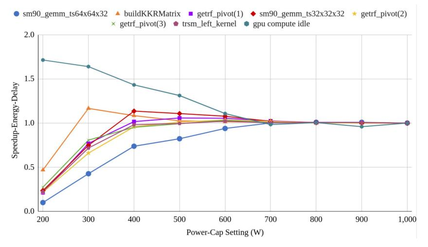
Speedup-energy-delay per GPU task and power-cap setting. Higher is better.
