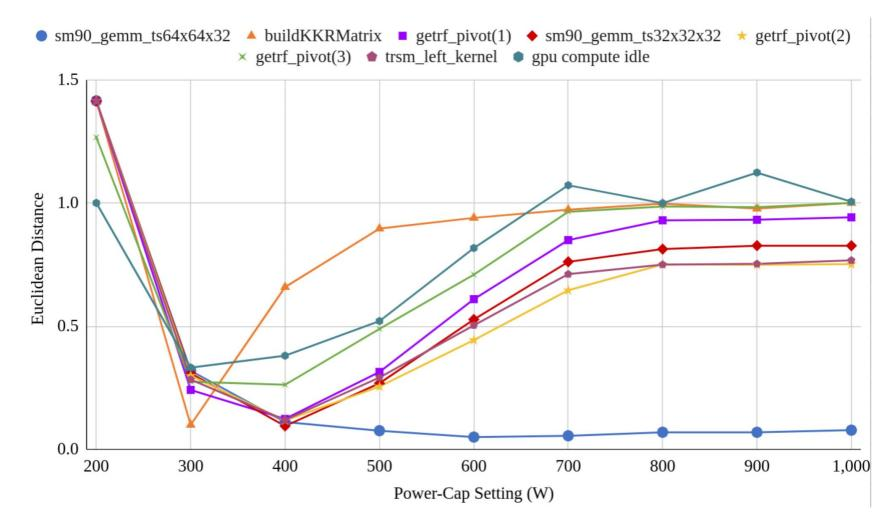
Euclidean distance of normalized energy/runtime per GPU task and power-cap setting. Lower is better.
