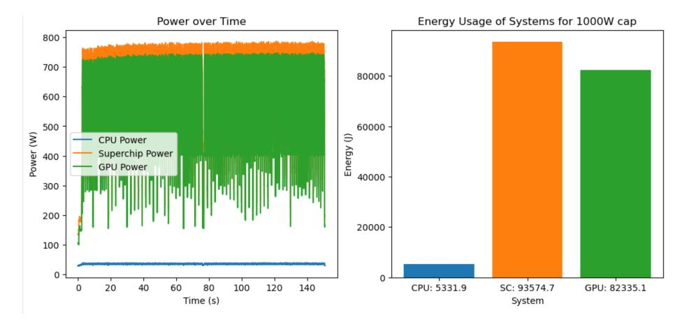
Power and total energy consumption, including CPU and GPU components (no power capping).
