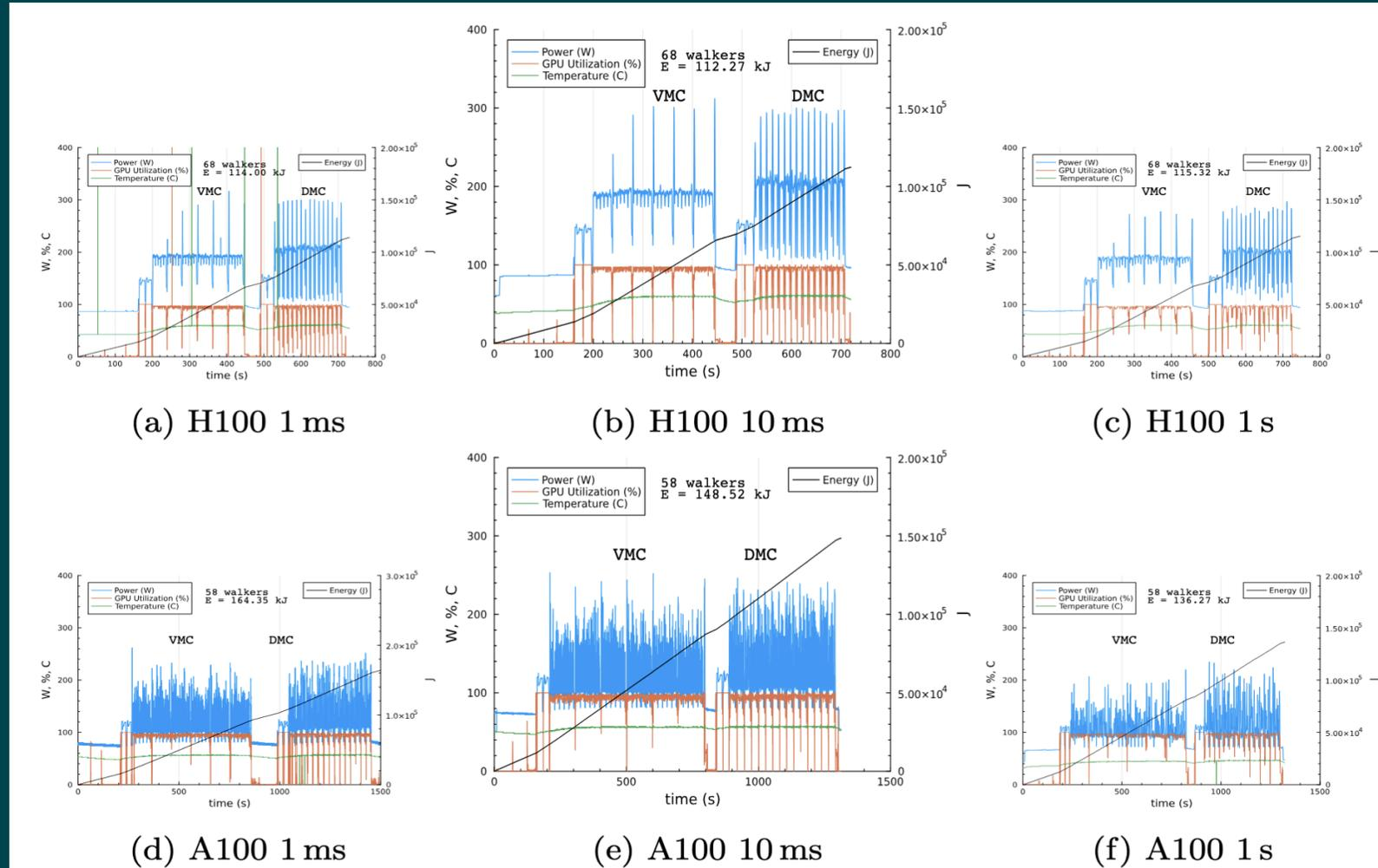
Fig. 2: Energy characteristics of the QMCPACK NiO benchmark on NVIDIA H100 and A100 for different query time resolutions.
