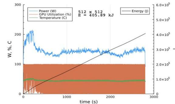
Fig. 8: AMReX-Castro Sedov energy characteristics on an AMD MI250X for a  $512 \times 512$  base mesh using double precision, 1 ms resolution, and CFL = 0.25.
