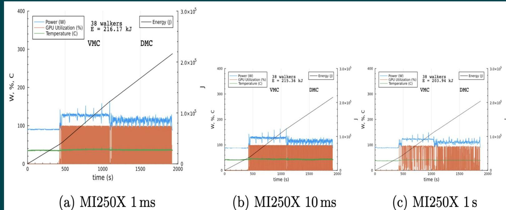
Fig. 3: Energy characteristics of the QMCPACK NiO benchmark on an AMD MI250X for different query time resolutions.
