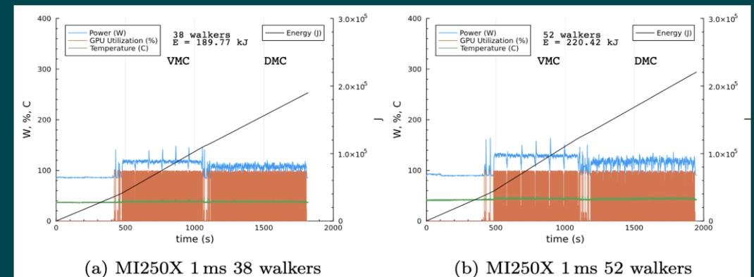
Fig. 5: AMD MI250X mixed-precision traces for (a) max double-precision walkers (38) and (b) max mixed-precision walkers (52).
